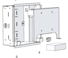
The P-TS18-WM wall mounting kit includes a recessed backbox, touchscreen mounting bracket, RJ45 punch down Ethernet connector, two foot Ethernet extension cable, and a terminal block for AC input termination.
