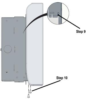
Step 10: Secure the touchscreen in place using two screws (provided in the wall mounting kit) through the bottom of the backbox to the mounting bracket (see graphic above).
